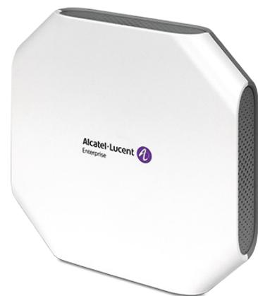
The efficient 802.11ac AP1201 access point supports a maximum concurrent data rate of 1.2 Gb/s (867 Mb/s in 5 GHz and 400 Mb/s in 2.4 GHz), 80 MHz channels (VHT80), multi-user MIMO (MU-MIMO) and two spatial streams (2SS) per radio. It provides simultaneous multicast data transmission to multiple devices, maximizing data throughput and improving network efficiency.
